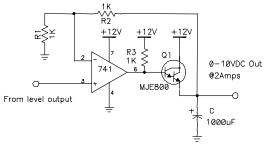
This configuration allows a user to adjust a 12VDC-18VDC unregulated power supply to a 0-10VDC regulated supply. The regulation in this case is limited to how well the URC1's regulator is operating. Parts can be modified in value to
